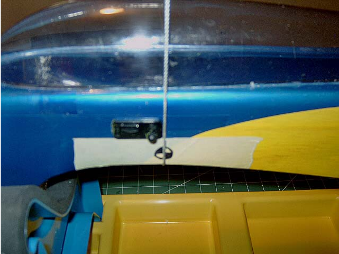
I ran the sting under the wing saddle with the string centered on the C.G. location.
